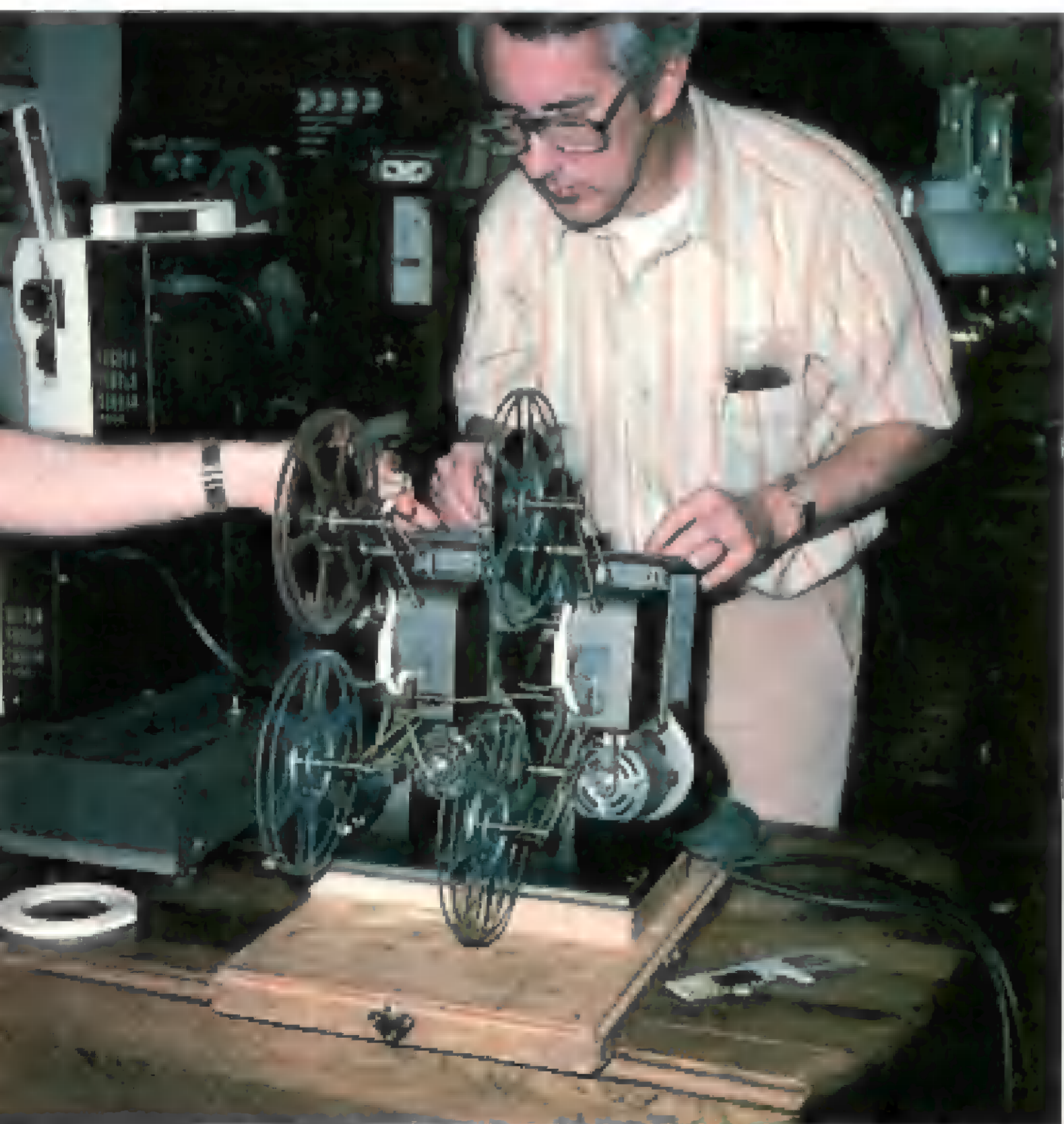
John Hart prepares to screen a dual 8mm 3-D film with a pair of mechanically interlocked Kodak projectors—a custom-built rig.
